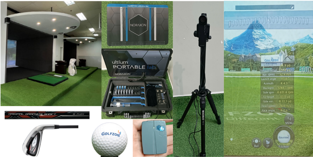
Fig. 1. Experimental setup including Noraxon Ultium Portable Lab , IMU sensor placement, Golfzon Vision system, 7-Iron Club, NiNox 120fps Camera
